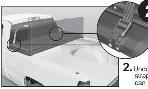
**2.** Undo both tie-down straps so cover can be unfolded.
