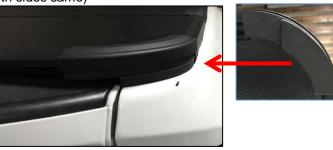
(3) After adding the foam, we need to put the 5mm foam strip on the truck to fullfil the gap. The 5mm foam strip should be put along the inner edge of the truck.
