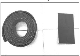
(1) The seal on above photo (L), put it on tailgate door. (As the photo shows below)
