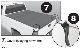
**8a**. Secure tailgate clamp hooks for a snug fit.
