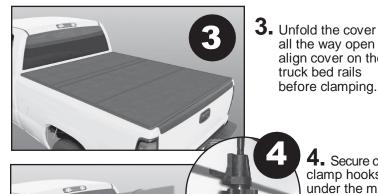
**4.** Secure cab clamp hooks under the metal bed rail. **Toyota Models** Only - Tighten lock nut at bottom of knob.
