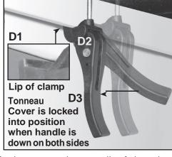
${f 8b}$ . To clamp cover down, put lip of clamp hooks under the side metal bed rail and push handle down. (See D1, D2, D3)
