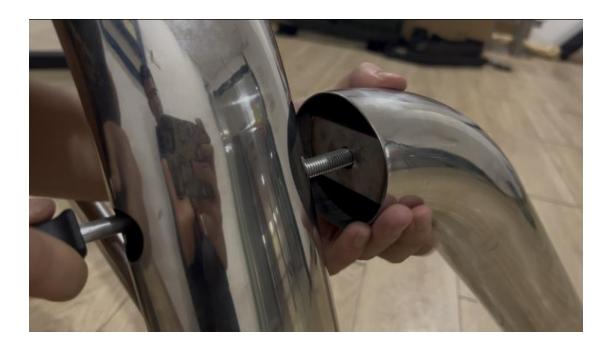
1. When the screw throw the hole, you don't need so tighten it so tightly, make sure it can intall the plastic part and bracket, you can tighten the pipe when you install the plastic part.
