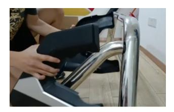
2. Put the screws we have prepared onto the corresponding holes
