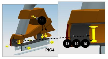
Step 4: Install (7) (8) Metal Base to the main body as shown in Picure 4.
