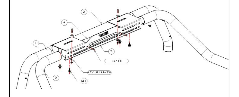
Connect decoration plates with the front tube and rear tube.
