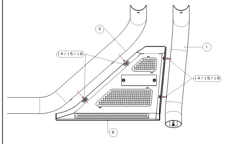
Install the roll bar on the vehicle shown as below.
