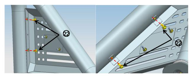
Step 6: Install 9 10 11 12 by 13 and lock it with the installed bar.
