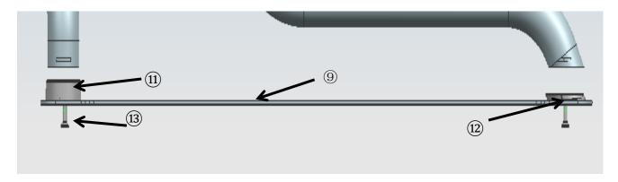
Step 7: Place the installed roll bar on the trunk of the truck and adjust it to a suitable position, then use 4151617 to fix 9 on the bodywork, and fix and lock the roll bar.
