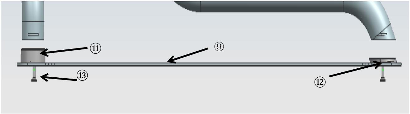
Step 7: Place the installed roll bar on the trunk of the truck and adjust it to a suitable position, then use ⑭⑮⑯⑰ to fix ⑨ on the bodywork, and fix and lock the roll bar.
