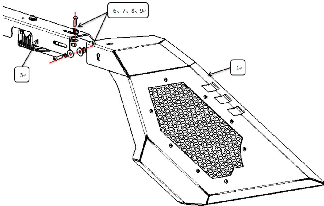
**Step 3:** Connect brackets and roll bar with standard parts ①⑥ ①⑧ ①⑨ ②① as figure shows.
