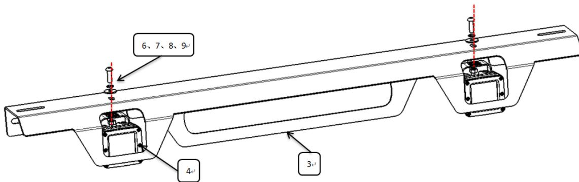
**Step2:** Install ① ② ③ and ④ with ⑥ ⑦ ⑧ ⑨ as below diagram shows.
