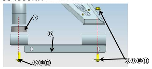
Step4: Place the installed roll bar on the trunk of the truck and adjust it to a suitable position, then Page 4 of 5
