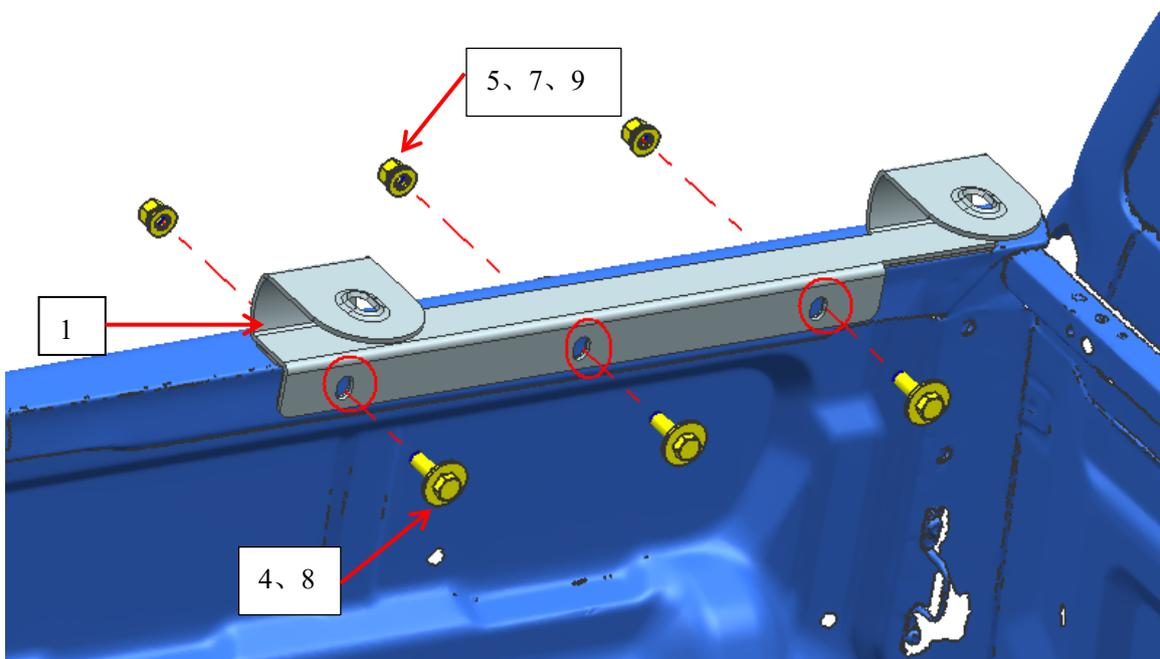
Step 3: Install MR Roll Bar on the brackets.
