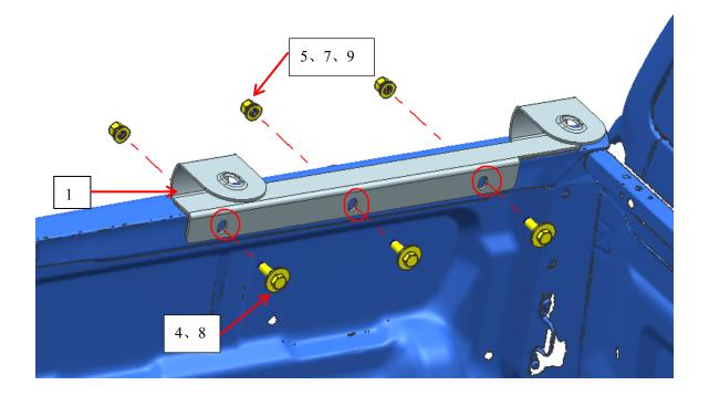
Step 3: Install MR Roll Bar on the brackets.
