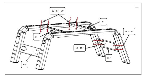
**STEP 4:** Connect cargo rack and FB roll bar with Front & Rear longitudinal beam (1) by using (16) (17) (18), adjust to the appropriate position and tighten all standard parts.
