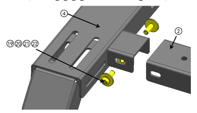
Step4: Using hardware (9)(2)(2)(2) to install Side beam (1), Longitudinal beam (1) and Support base (2)(6)(7), do not tighten all the hardware.
