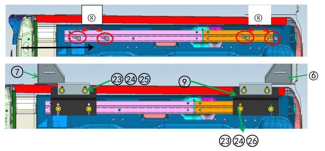
Step 5.2 (RANGER): Use hardware (4) (2) (2) (9) to install TRUCK BED RACK on the truck, do not tighten all the hardware.
