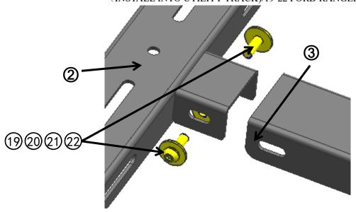
Step 3: Using hardware 19202122 to connect Cross beam and Longitudinal beam 2.
