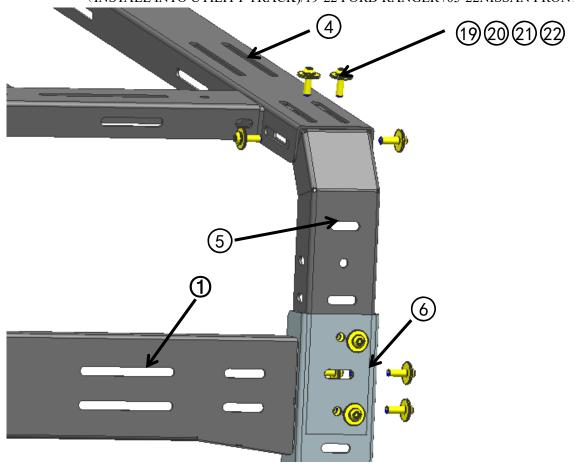
Step 5.1 (FRONTIER): Slide Nut plates 8 in the truck, and then use hardware 3 2 4 2 to connect 9 with 8. Use hardware 3 2 4 25 to install 9 with 6/7, do not tighten all the hardware.
