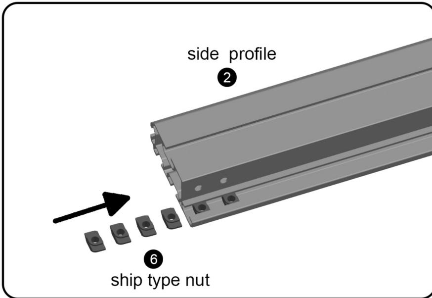
Match the number of standard flat , and then insert the ship type nuts with the same number as the standard Flat into the chute of the side profile.
