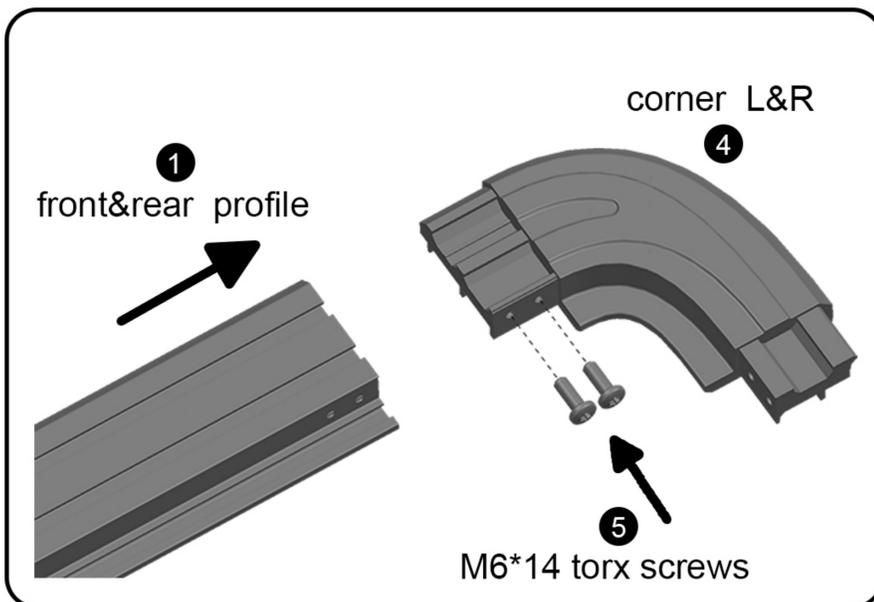
Insert the corner into the front&rear profiles and screw in the Torx screws.
