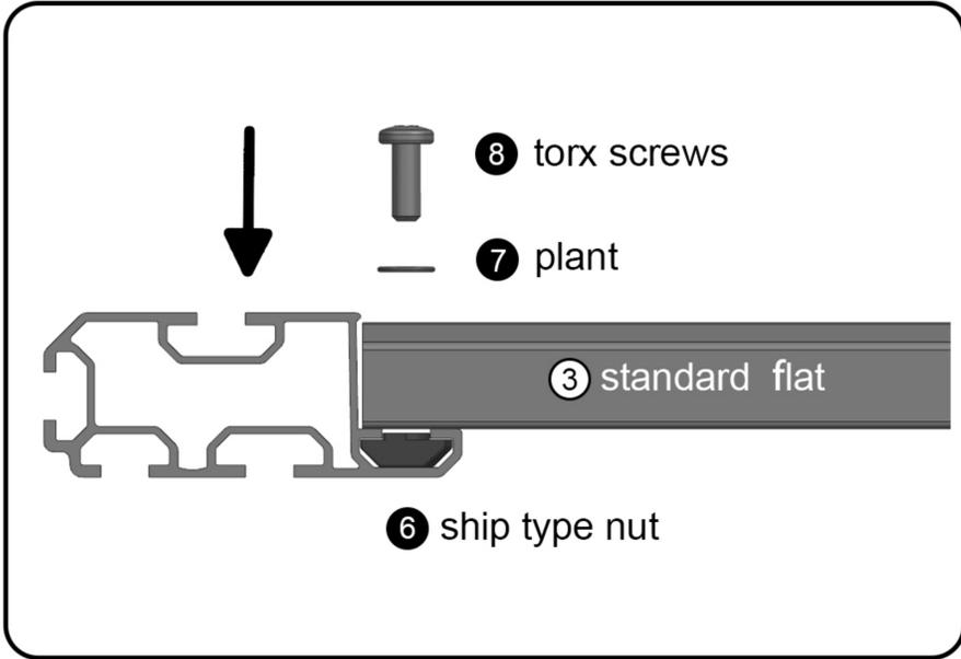
Place the standard flat on the side profile, and use screws and ship type nuts to lock the standard flat on the side profile.
