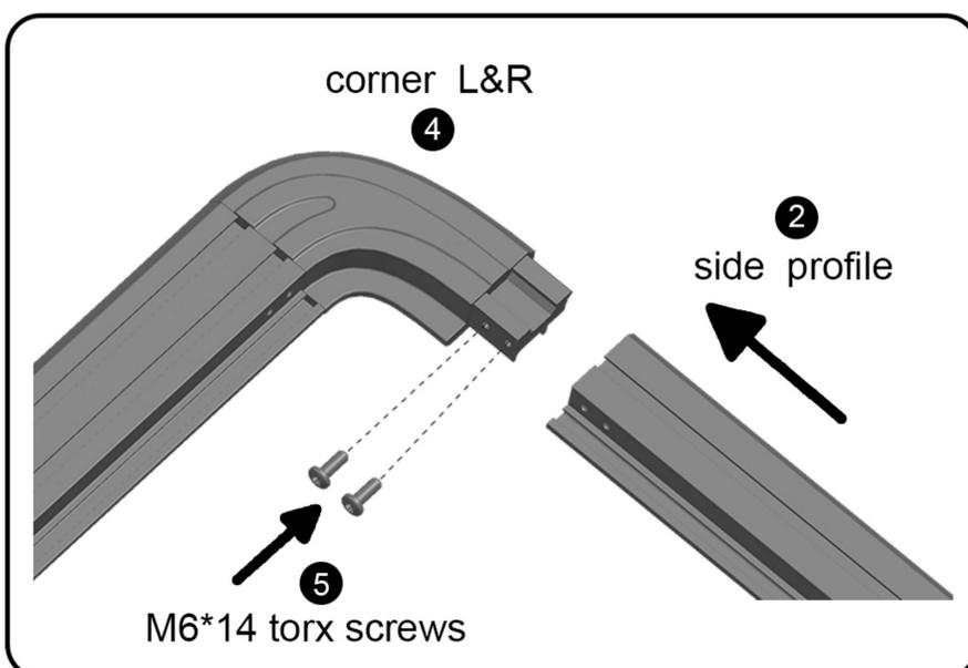
Insert the corner into the side profiles and screw in the Torx screws.
