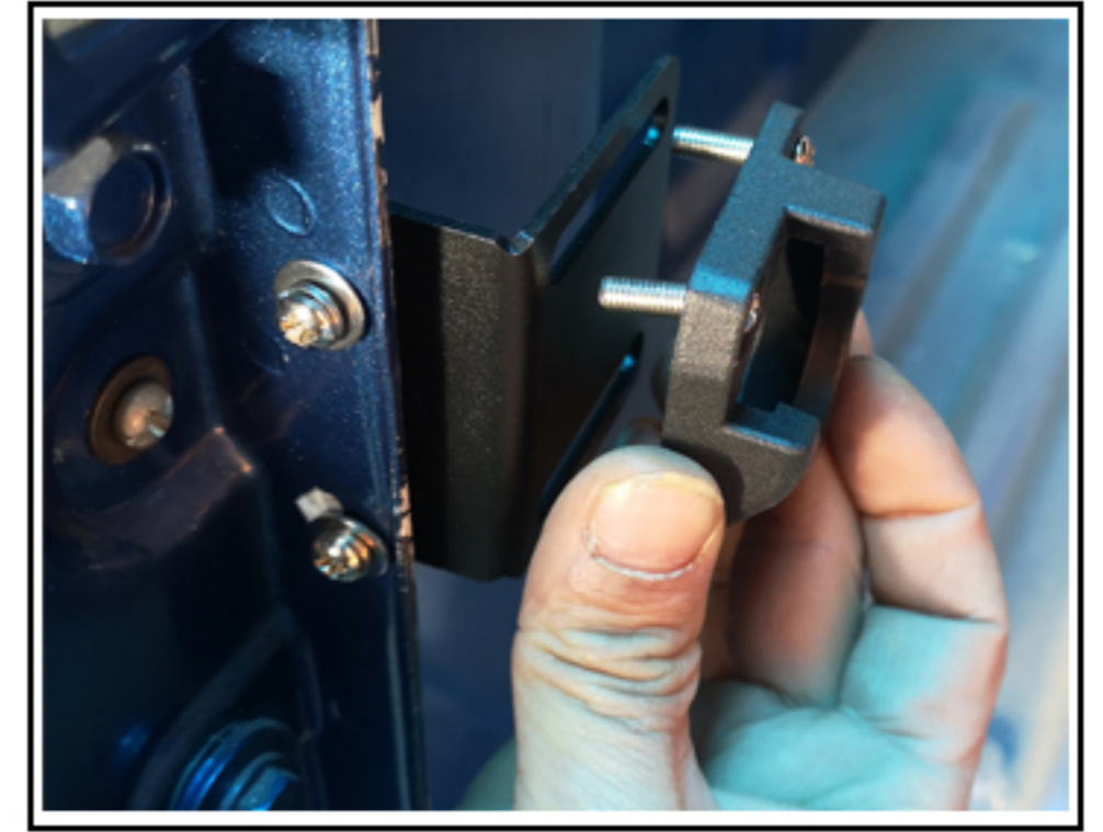
13. As shown in the figure, match bracket 2 to the hole of bracket 1, and insert the screw.
