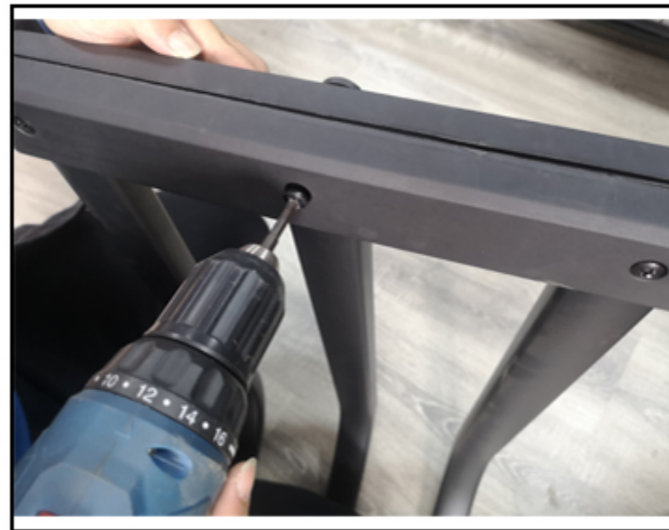
8. As shown in the picture, Match the other half of the bracket to the hole, use an electric drill to tighten the middle screw
