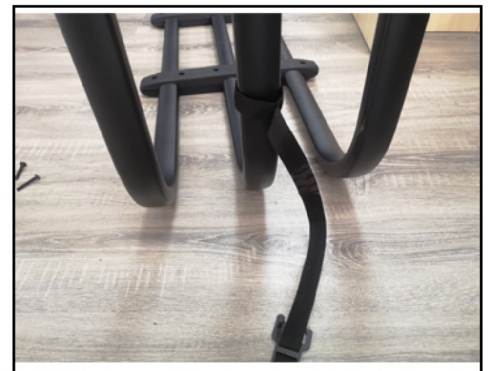
6. Pass the rope into the middle elbow and do the same at the other end
