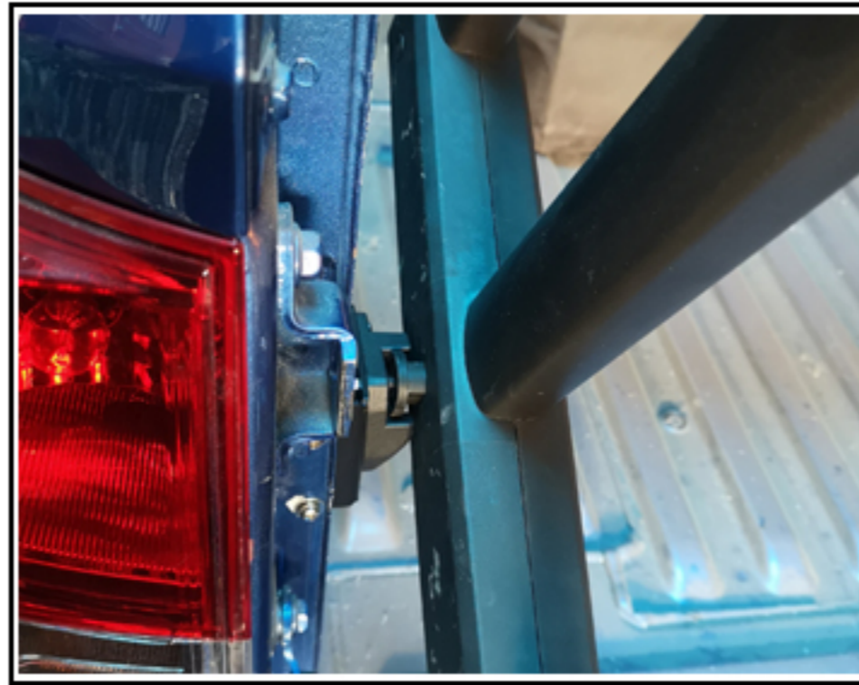
15. As shown in the figure, erect the expansion frame, and the side corresponds to the bracket 2.
