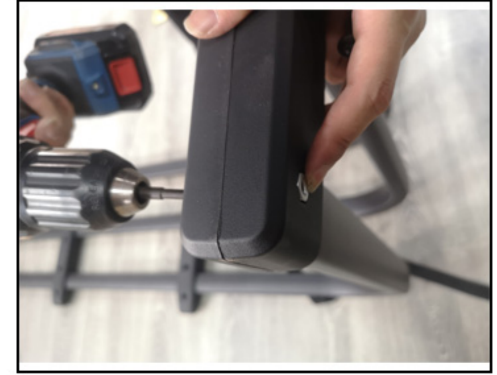
9. As shown in the picture, put the nut on the outside and tighten the screw on the inside
