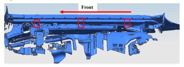
Install the bracket on the original car in turn, and then adjust the side step to a suitable position to install with the bracket, and the left and right are consistent.
