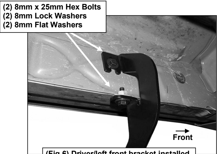
(Fig 6) Driver/left front bracket installed
