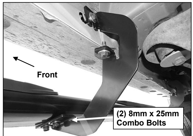
(Fig 20) Passenger/right center bracket installed
