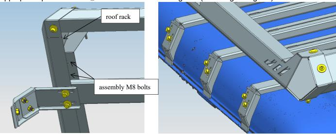
Step 3: According to the INSTALLATION PICTURE, assemble the ③bracket 3 to cover the outside edge of rain gutter (see the picture below).
