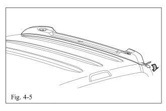
(g) Align the stub on the rear of the pad with the roof ditch, once aligned, remove tape backing and press down firmly. Tuck the stub under the rear window lace. (Fig. 4-5)
