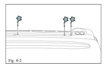
(d) Hand start the 3 long torx head screws into roof rack along roof ditch. (Fig. 4-2)
