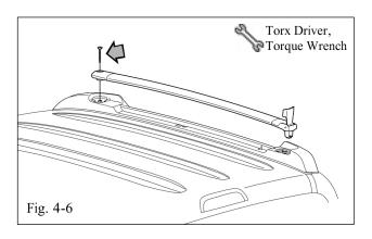
(h) Install crossbar assembly to roof rack. (Fig. 4-6)
